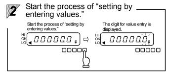
Press the bound key, and the process of setting by entering values" is enabled with all digits displayed. Only the LSD blinks, indicating that it is the digit for value entry.
