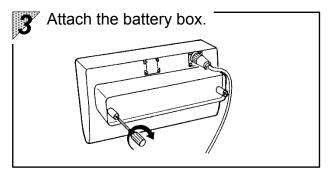
Connect the relay connector of the battery box and install it on the display.
