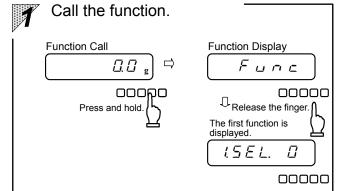
Press and hold the seven for approximately 4 seconds. When "Func" is displayed, release the
