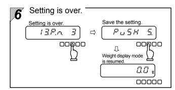
Press the  $\bigoplus_{sar}$  key, and the setting is saved and " $P \sqcup 5 H$  5." is displayed.
