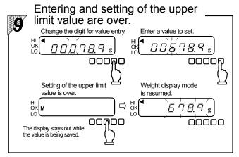
As in the case of entering the lower limit value, select the digit for value entry with the key and select a value to set with the weak key for entry of the upper limit value.
