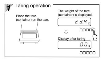
Place the tare (container) on the pan and press the  $\frac{1}{300 \text{ TeV}}$  key, and the readout changes to zero.  $\Rightarrow$  Refer to "Taring."
