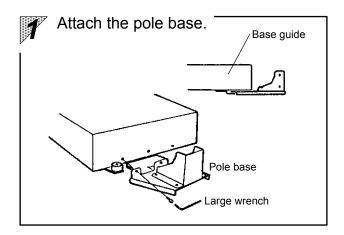
Install the accessory pole base to the base guide at the bottom of the scale with the supplied large wrench. Unless the pole base fits the guide correctly, the pole base cannot be installed on the scale.
