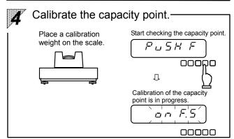
Gently place a calibration weight at the center of the pan.
