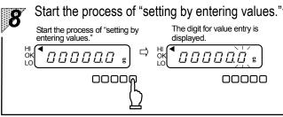
Press the bound key, and the process of setting by entering values' is enabled with all digits displayed. Only the LSD blinks, indicating that it is the digit for value entry.
