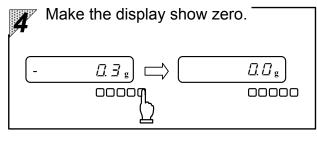
If the display readout does not become zero, press the →07+ key to make the display show zero. ⇒ Refer to "Set the zero point."
