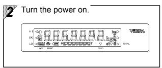
At this time, check that no LEDs nor LED segments stay out.
