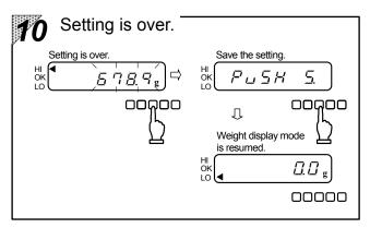
Press the key, and the set value is saved and "Fush key again, and the setting process is terminated and the weight display mode is resumed.
