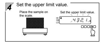
Place the sample for the upper limit value on the scale and press the  $\[\Box\]$  key.
