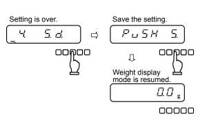
Press the  $\frac{\textcircled{*}}{\sec}$  key, and the setting is saved and " $P \sqcup \underline{S} H = \underline{S}$ ." is displayed.
