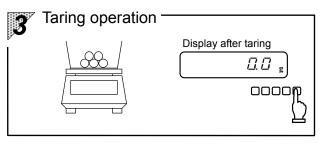
Press the  $\frac{90 \text{ Te}}{2\pi n \text{ Ter}}$  key, and the readout changes to zero.  $\Rightarrow$  Refer to "Taring."
