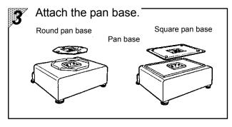
Set the pan base with its screw hole aligned to the projection on the main body and tighten the screw with a screwdriver or an appropriate coin.
