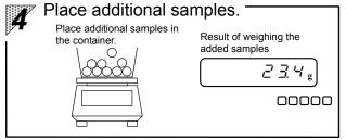
When additional samples are placed in the container, the weight of only the added samples is displayed.
