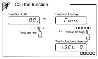
Press and hold the  $\Box$  key for approximately 4 seconds. When " $F \ \sqcup \ \cap \ \varepsilon$ " is displayed, release the
