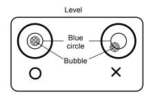
Rotate the four adjusters until the bubble in the level fits within the blue circle.
