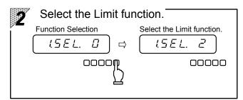
Press the  $\frac{90\%}{\text{leavin}}$  key, and the rightmost value changes. Then select the limit function "Z".
