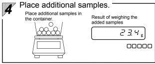
When additional samples are placed in the container, the weight of only the added samples is displayed.
