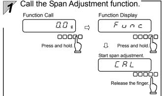
Press and hold the fraction key until the display changes from "F , r , r , r " to " [ R ] " to enter the Span Adjustment mode. (This will take approximately 6 seconds.)
