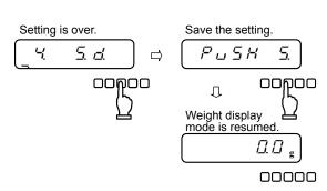
Press the weight key again, and the setting process is terminated and the weight display mode is resumed.
