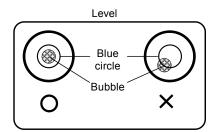
Rotate the four adjusters until the bubble in the level fits within the blue circle.
