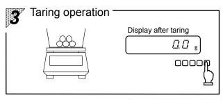
Press the  $\frac{|\neg 0.74|}{|\neg 0.74|}$  key, and the readout changes to zero.  $\Rightarrow$  Refer to "Taring."
