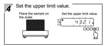
Place the sample for the upper limit value on the scale and press the [s] key.
