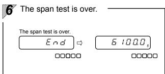
When the adjustment of the capacity point is over, the weight display mode is resumed after " $E \cap I$ " is displayed, indicating that the span adjustment is completed.
