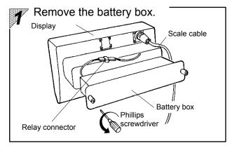
Loosen the screw in the rear of the display and the battery box can be removed.
