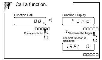
Press and hold the seven for approximately 4 seconds. When "Func" is displayed, release the fineer.
