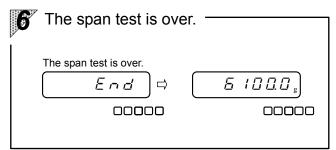
When checking of the capacity point is over, the weight display mode is resumed after " $E \cap I$ " is displayed, indicating that the span test is completed.
