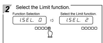
Press the  $\frac{90\%}{\text{lawler}}$  key, and the rightmost value changes. Then select the limit function " $\vec{c}$ ".
