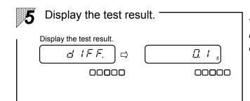
When checking of the capacity point is over, the test result is displayed in terms of weight after "d' 1 F F." is displayed.
