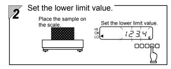
The display disappears temporarily. When the lower limit value is saved, the display blinks.
