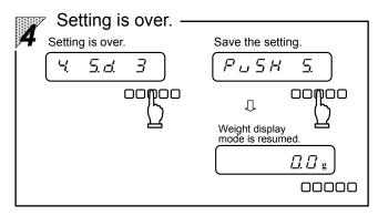
Press the key, and the setting is saved and "P \( \omega \) 5 \( H \) 5." is displayed.
