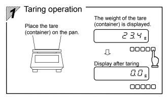
Place the tare (container) on the pan and press the  $\frac{1}{\log n}$  key, and the readout changes to zero.  $\Rightarrow$  Refer to "Taring."
