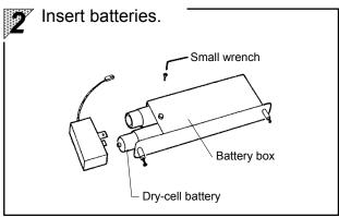
Remove the battery box cover with the small wrench in the accessory kit.
