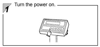
Press the wey on the panel, and all the indicators light up, showing that the instrument is operating.
