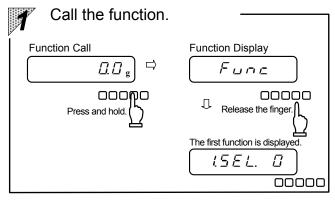
Press and hold the  $\frac{\Box}{\Box}$  key for approximately 4 seconds. When " $F \ \Box \ \cap \ \Box$ " is displayed, release the
