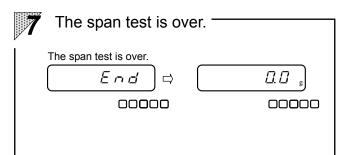
When checking of the capacity point is over, the weight display mode is resumed after " $E \cap d$ " is displayed, indicating that the span test is completed.
