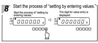
Press the book key, and the process of setting by entering values" is enabled with all digits displayed. Only the LSD blinks, indicating that it is the digit for value entry.
