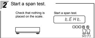
Check that nothing is placed on the pan. Press the key while holding the key down and then release the keys simultaneously. "E, E H E." is displayed and a span test is started.
