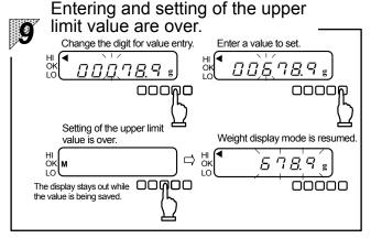
As in the case of entering the lower limit value, select the digit for value entry with the key and select a value to set with the wear key for entry of the upper limit value.
