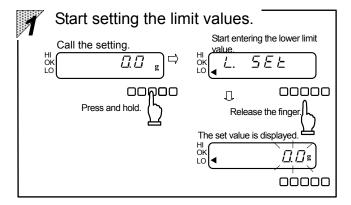
Press and hold the well key for approximately 3 seconds. When
