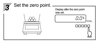
When additional samples are placed in the container, press the house key so that zero is shown in the display.
