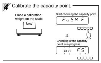
Gently place a calibration weight at the center of the pan.
