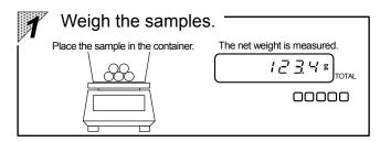
Place samples on the scale for weighing.
