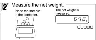
When samples are placed in the container, the net weight of the sample is displayed.
