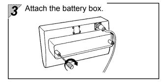
Connect the relay connector of the battery box and install it on the display.
