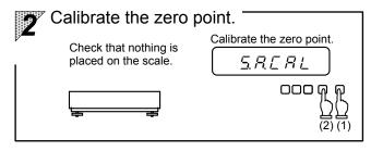
Check that nothing is placed on the pan. Press the holding the key while holding the key down and then release the keys simultaneously. "5. R. [ R ]." is displayed and span adjustment is started.
