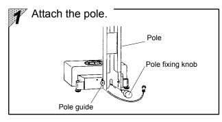
Install the accessory pole to the rear guide with the pole knob.
