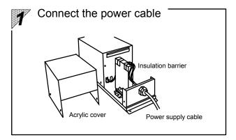
Remove the acrylic cover and connect the power cable.
