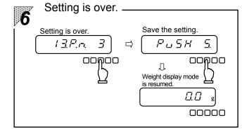
Press the \$ key, and the setting is saved and " $P \cup S H \subseteq S$ ." is displayed.
