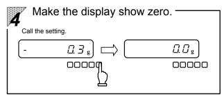
If the display readout does not become zero, press the  $\frac{1}{200 \text{ Te}}$  key to make the display show zero.  $\Rightarrow$  Refer to "Set the zero point."
