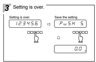
When the setting is over, press the \$ key, and the setting is saved and  $\textcircled{\$P} \sqcup 5 H \_ 5$ ." is displayed.
