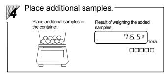
When additional samples are placed in the container, the weight of only the added samples is displayed.
