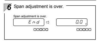
When the adjustment of the capacity point is over, the weight display mode is resumed after " $E \cap d$ " is displayed, indicating that the span adjustment is completed.
