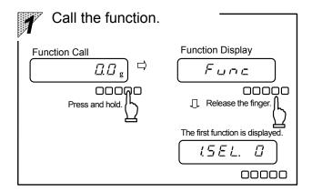
Press and hold the provided Rey for approximately 4 seconds. When " $F \sqcup \neg \subset$ " is displayed, release the finger. Now the function setting mode is assumed and the first item " $L \subseteq E \sqcup \square$ " (Function Selection) is displayed.
