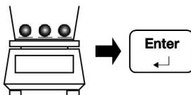
Remove the object to be weighed. After 「 \* 」 appears, push [Enter] key.
