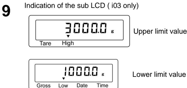
The upper and lower limit values that have been set are indicated on the sub LCD.
