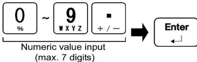
Input a tare weight value with the [Numeric keypad].
