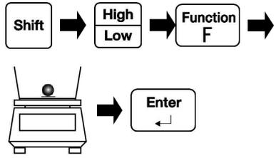
Push the [Shift] key and the [High / Low] key in the scale mode.
