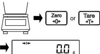
Remove the tare and the object to be weighed from the weighing pan.
