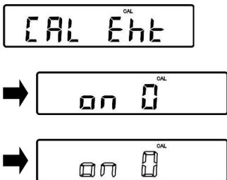
The indication changes to the flashing of "CAL EHT", "on 0", and then "on 0", followed by the starting of the zero-point adjustment.
