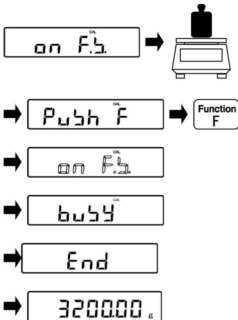
After completion of the zero-point adjustment and the indication changing to "on F.S.", place the weight in the center of the weighing pan. The indication changes to "PUSH F".
