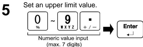
Input an upper limit value with [Numeric keypad].
