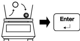
Remove the previous object to be weighed to return the indication to zero and then place a next object to be weighed.
