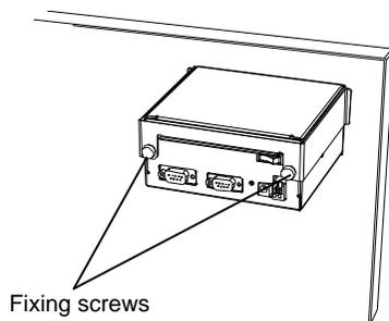
Tighten the clamping screws manually. Check that the indicator is clamped securely.
