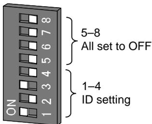
Switches No. 1 to 4 are used to set an ID number.
