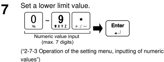
Input a lower limit value with [Numeric keypad].
