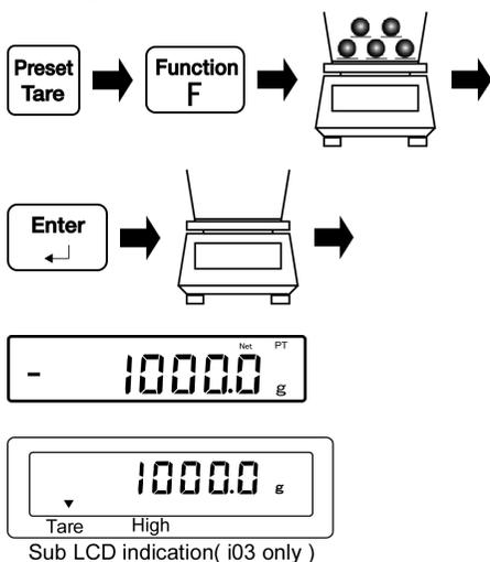
**2** To exit the preset tare weight subtraction mode
