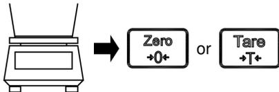
Remove the tare and the object to be weighed from the weighing pan.
