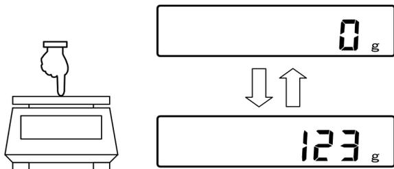
Press the weighing pan lightly to check if the indication changes.
