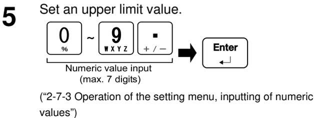
Input an upper limit value with [Numeric keypad].
