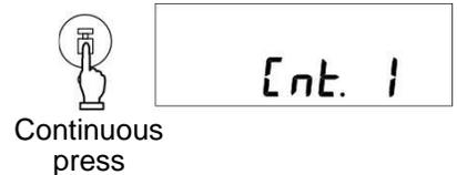
After a while, the display switches to [Cnt. 1] and the measurement starts. As the repeatability measurement proceeds, the number of measurements displayed in [Cnt. \*] increases accordingly until it reaches [10].
