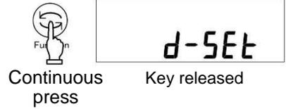
Press the **Function** key to display the clock time and press the **Function** key again. The display automatically indicates a date after indicating [dAtE].
