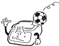
◆ **Avoid applying excess force or impact to the balance.**
