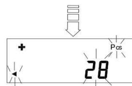
Repeating this operation will improve the resolution of parts counting for more accurate measurements.
