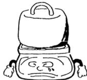
◆ **Do not leave the balance overloaded. (When it is overloaded, (o-Err) is displayed.)**
