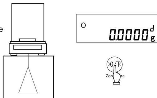
4. Measure the weight of the sample in the air.
