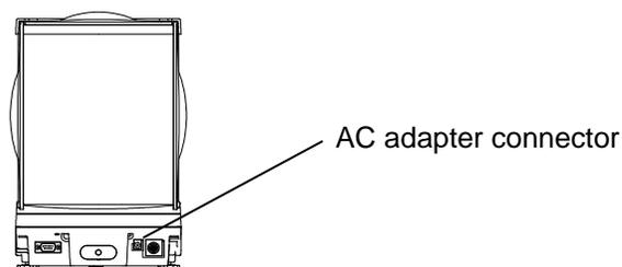
After the balance has been moved, open the windshield door to allow it to adapt to the ambient temperature for stable measurement.
