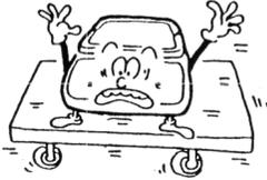
◆ **Do not place the balance on an unstable base or use the balance in a location where it may be subjected to shock.**
