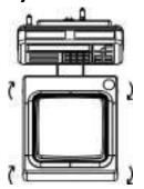
At the time of shipment, the adjusters provided at the four corners of the bottom are locked. Turn them in the direction shown in the figure on the left to loosen them.
