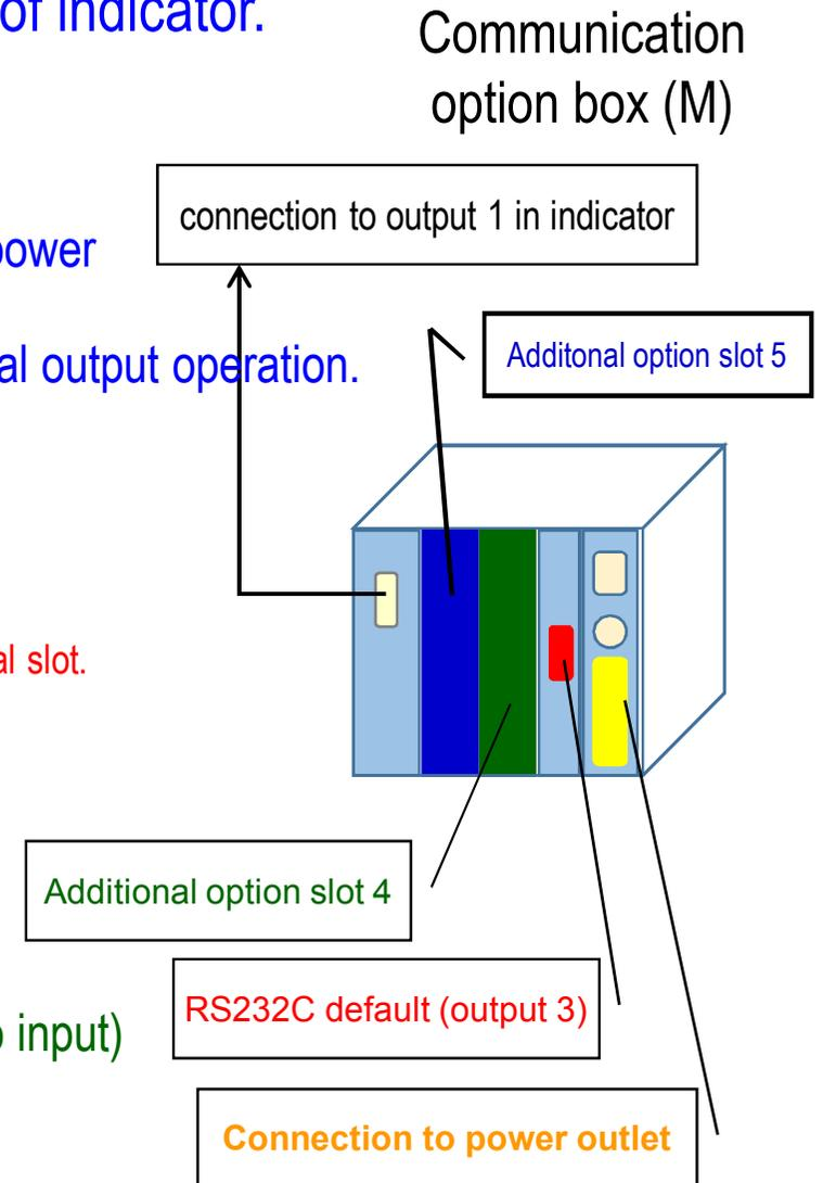
Additional option slot 5: Relay contact (FS-LM) can be installed here.
