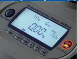
Red alert signal is blinking during heating process. You can immediately notice when the measurement is completed.
