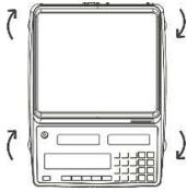
At the time of shipment, the adjusters provided at the four corners of the bottom are locked. Turn them in the direction shown in the figure on the left to loosen them.
